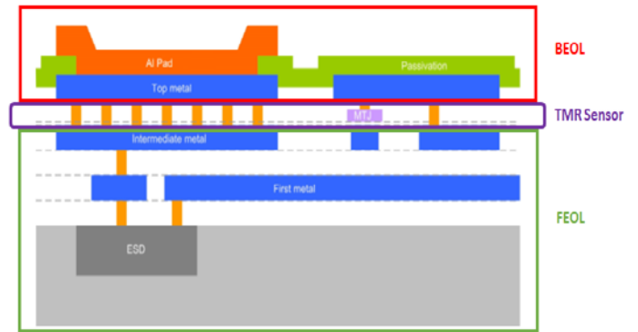
Figure 12 Typical CMOS structure.
