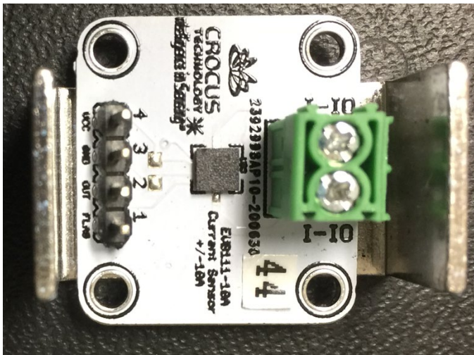
Figure 7. EVB111 with a U-shape shield.
