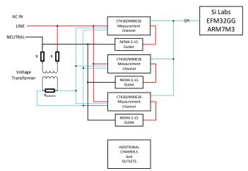
Figure 2: PDU Demonstration Board Block Diagram
