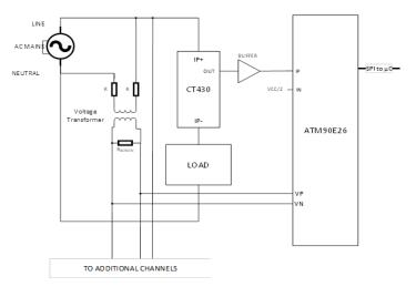
Figure 1: PDU Channel Architecture
