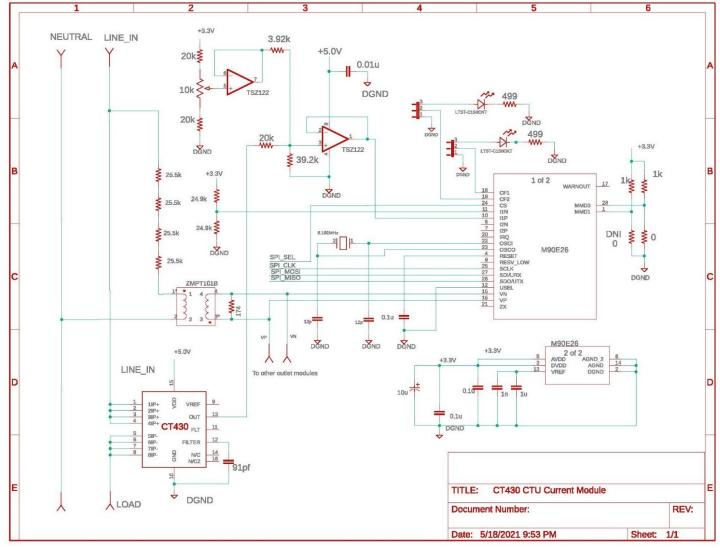
Figure 6: CT430 PDU Outlet Module
