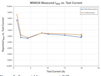
Figure 5: Current Measurement Difference
