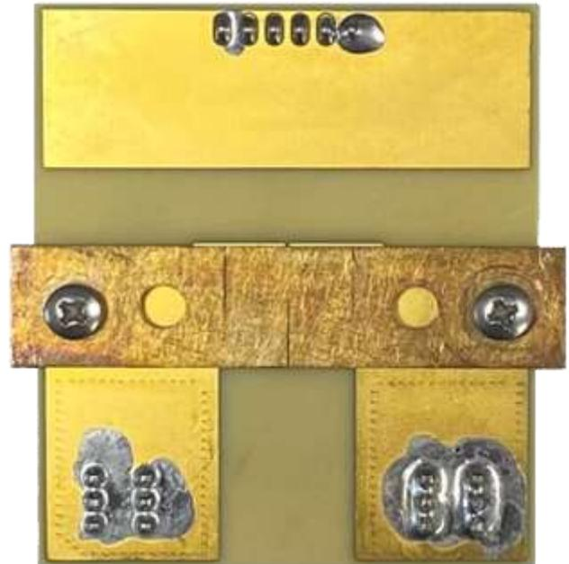
**Figure 6.** CTD452/3 with busbar mounted on the bottom
